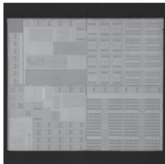
Inspect module integrity under IR 1300nm coaxial light
