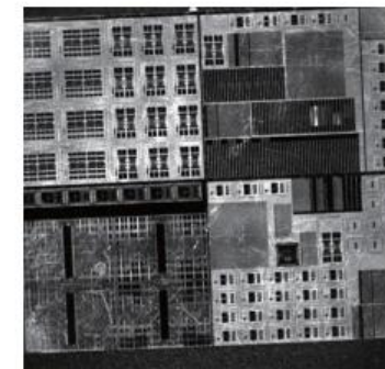
Detect surface scratches with white coaxial light
