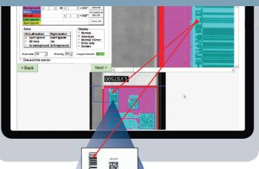
The LVS-7500 label inspection system provides 100% label inspection as labels are printed at production printing speeds. In the event of a label defect the printer is automatically stop ensuring that the defective label is confirmed by an operator and removed.
