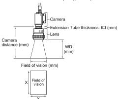
Note: 1. The lengths of the fields of vision given in the optical charts are the lengths of the Y axis.
