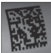
Data Matrix on Curved Surface
